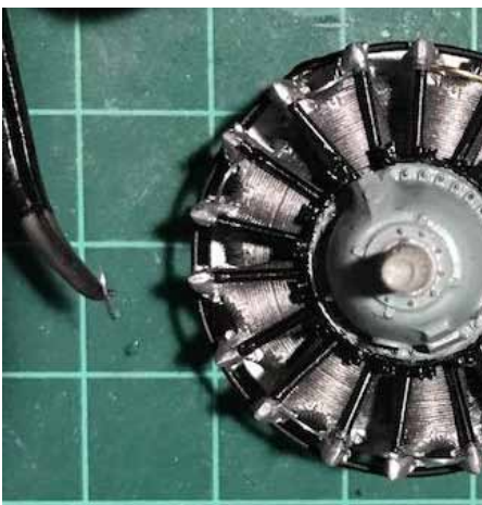
Figure 10: Arc-shaped pieces of 30-ga. wire connect the cylinder “ears”.
