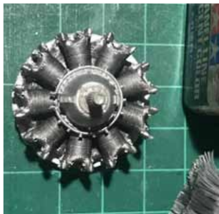
Figure 6: Black panel line accent wash applied to cylinders
